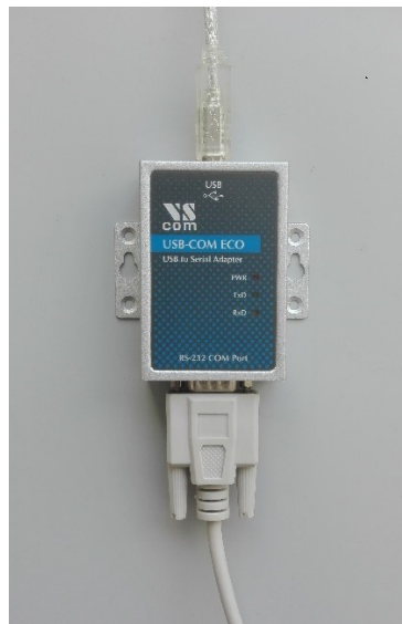
Fig. 3. Back panel of a ROXY Potentiostat (left) and VScom 1-port RS232-USB converter. Converter is connected to computer using an USB port.
